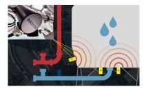
**HASYTECgroup** has developed a patented ultrasound intelligent technology to prevent deposits on all liquid-carrying surfaces. The innovative "Intelligent Deposit Protection®" IDP® Technology prevents biofilm accumulation and inorganic deposits in various industrial applications, such as cooling towers, plate/shell/tube heat exchangers, pasteurizers, bottle and plastic case washing machines, condensers, tanks, piping and many more.
